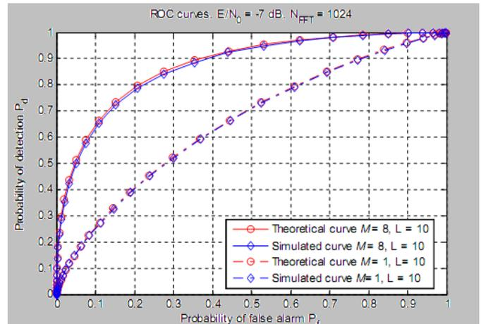
Figure 1:- Receiver operating characteristic. FFT = 1024, SNR = -7 dB
