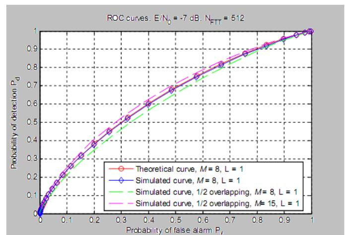
Figure 6:- Receiver operating characteristic. FFT = 512, SNR = -7 dB
