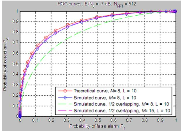
Figure 7:- Receiver operating characteristic. FFT = 512, SNR = -7 dB
