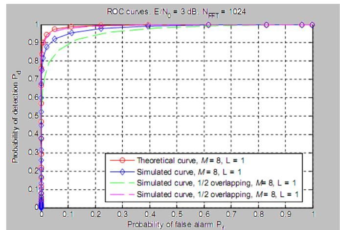
Figure 5:- Receiver operating characteristic. FFT = 1024, SNR = 3 dB
