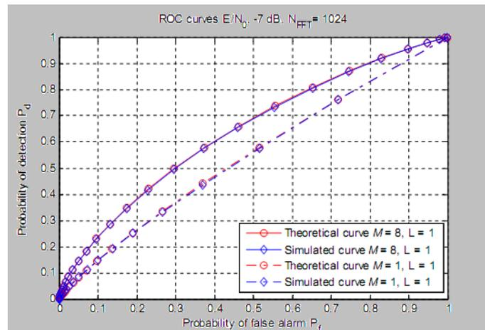
Figure 2:- Receiver operating characteristic. FFT = 1024, SNR = -7 dB
