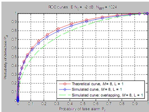
Figure 4:- Receiver operating characteristic. FFT = 1024, SNR = -2 dB
