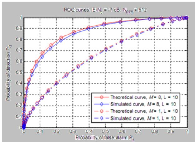
Figure 3:- Receiver operating characteristic. FFT = 512, SNR = -7 dB
