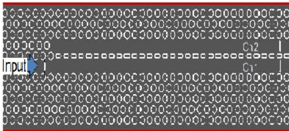
Fig. 6: The modified structure with rectangular air holes.
