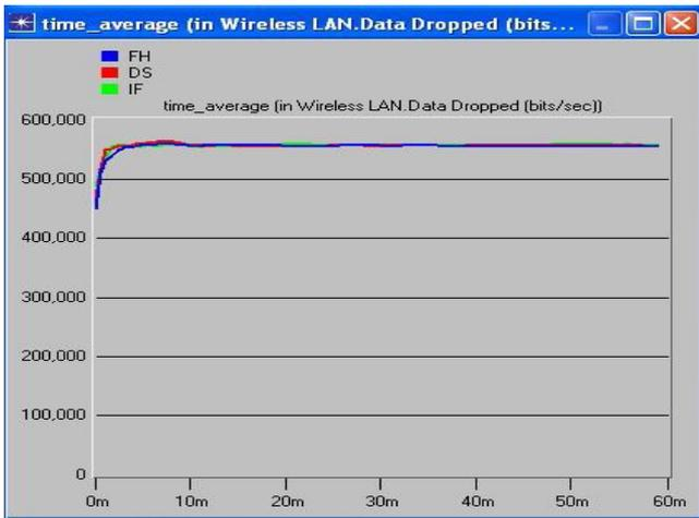
**Fig 3.3(c) Data dropped at 5.5 Mbps under different techniques**
