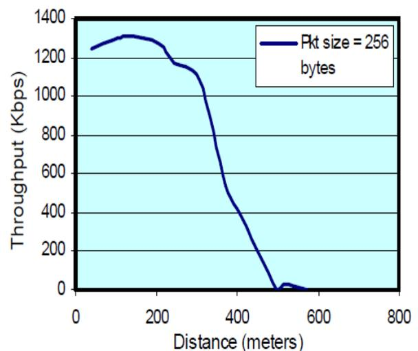
**Figure:3 Throughput vs Distance for Freeway Following Scenario**
