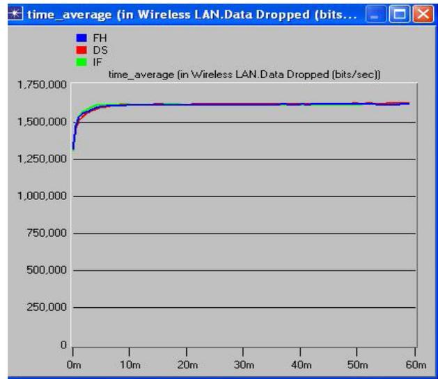
Fig 3.3(a) Data dropped at 1 Mbps under different techniques
