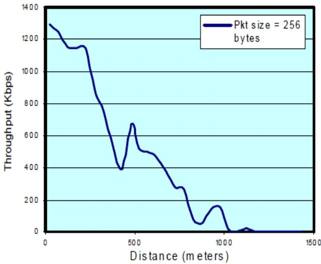
Figure:4 Throughput vs Distance for Suburban Scenario
