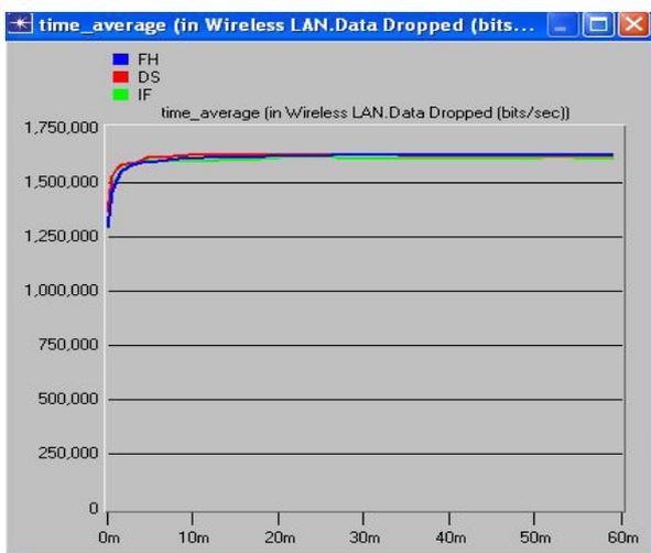
**Fig 3.3(d) Data dropped at 11 Mbps under different techniques**
