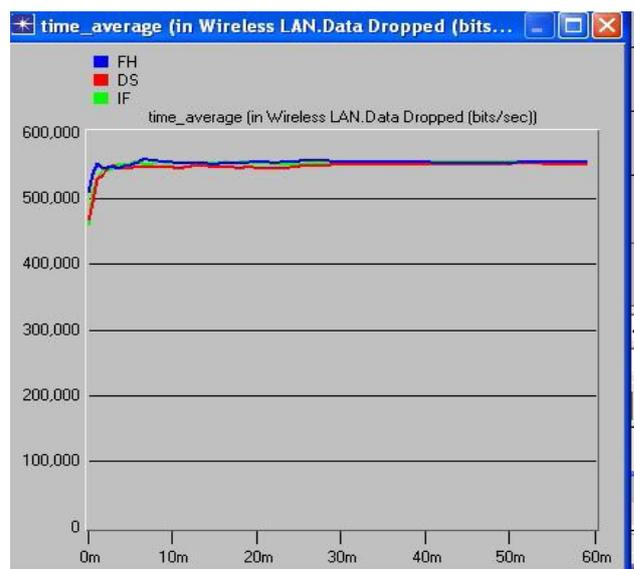
Fig 3.3(b) Data dropped at 2 Mbps under different techniques
