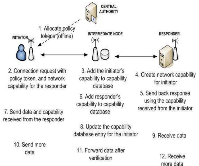
Fig1. MANET System Architecture
