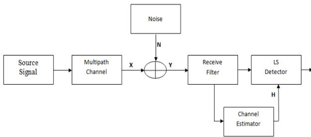
Figure 5: Block diagram of noise-corrupted LS Estimator
