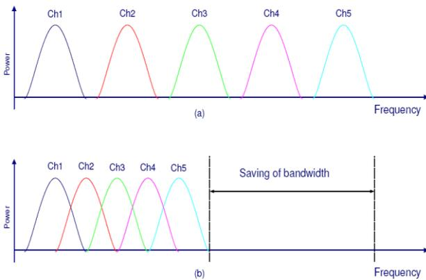
Figure 2 Concept of OFDM Signal: (a) conventional multicarrier technique (FDM) and (b) orthogonal frequency division multiplexing technique.
