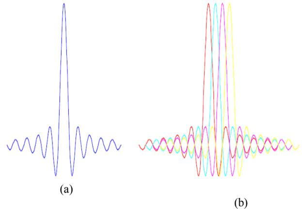
Figure 3 Spectra of an OFDM, (a) OFDM Sub-Channel (b) OFDM Symbol
