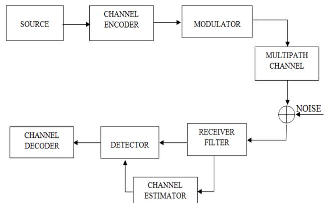
Figure 1 Block diagram of Channel Estimator
