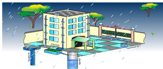
Fig 1.1 Rain Water Collection in Multi-Storied Building
