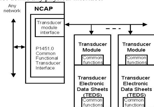
Figure.2 Block diagram of IEEE P1451.0
