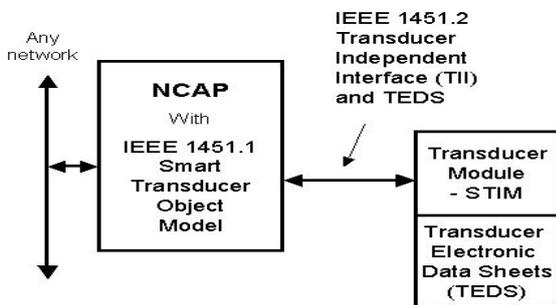
Figure 4 – System block of 1451.1 and 1451.2 interface to an integrated STIM.
