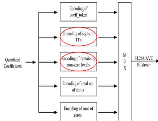
Fig. 3 Encircled syntax elements are used for SE-CAVLC [5].
