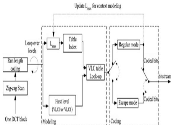
Fig. 2 Block diagram of level coding in CAVLC of H.264/AVC [5].
