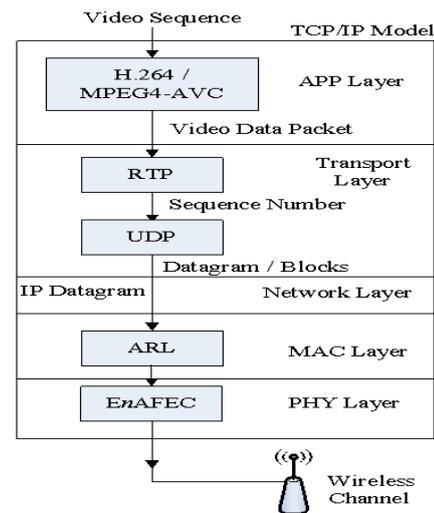
Fig. 7 Cross Layer Mechanism
