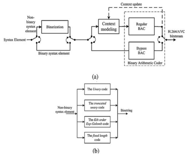
Fig. 4 (a) Block diagram of CABAC of H.264/AVC. (b) Binarization stage [5].
