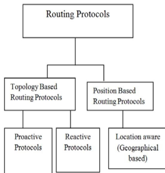
Fig1: Different Routing Protocols for Mobile Ad-Hoc Networks
