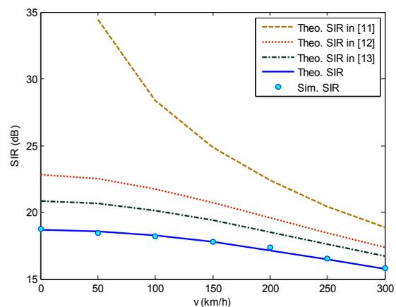
Fig. 1. SIR versus the NDF when  $\varepsilon = 0.05$  nd  $\beta T_s = 0.005$ .
