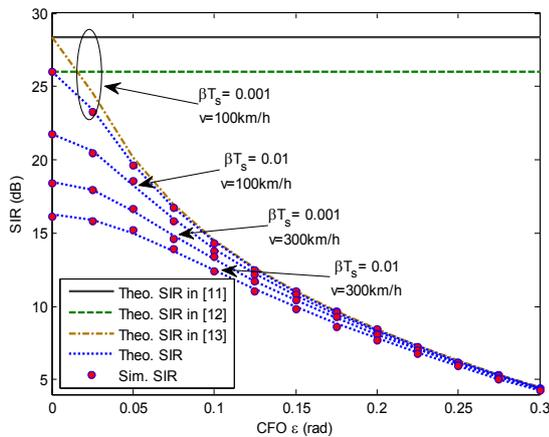
Fig. 2. SIR versus CFO when  $\beta T_s = 0.001$  and  $0.01$  under  $v = 100 \text{ km/h}$ .
