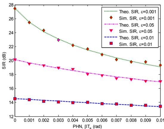
Fig.3. SIR versus PHN level  $\beta T_s$  under  $f_d T_s = 0.03$  ( $v = 100 \text{ km/h}$ ) and  $\varepsilon = 0.05, 0.01$ .
