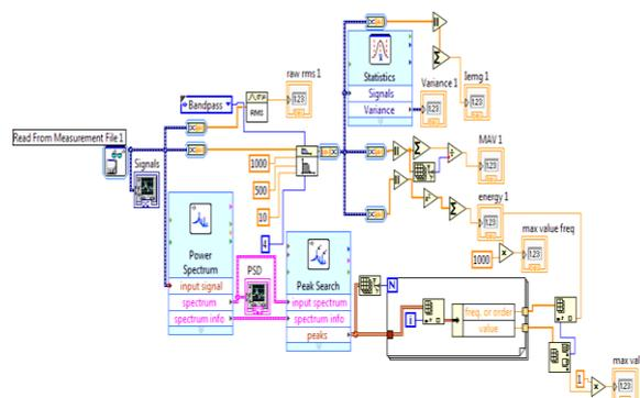
Fig. 2 Labview based code for feature extraction
