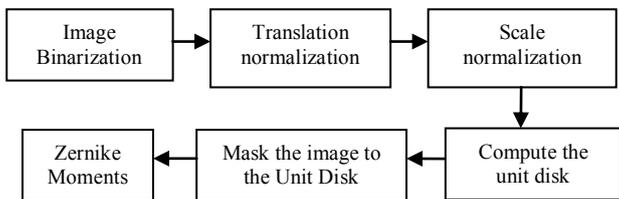
Fig. 4. Block diagram of computing Zernike moments.
