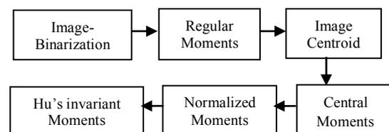
Fig.3 Block diagram of computing Hu's seven moment invariants.
