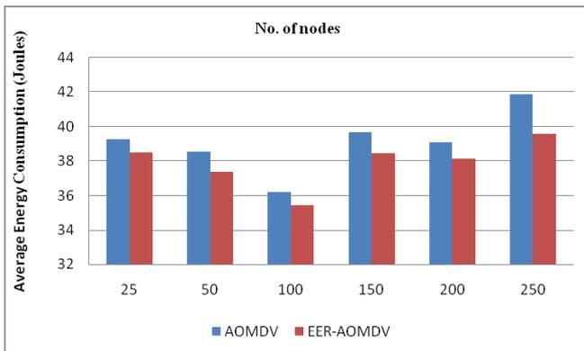
Fig. 2 Average energy consumption vs. no. of nodes
