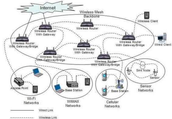
Fig. 2. Infrastructure/Backbone Architecture
