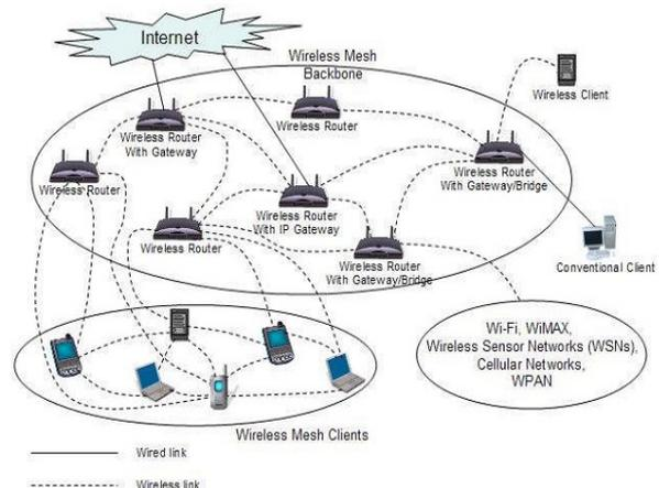
Fig. 3. Hybrid Architecture
