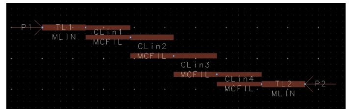
Fig. 7 Layout of parallel-coupled microstrip band pass filter.
