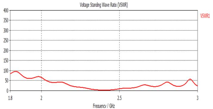
Fig.4. VSWR plot for the antenna
