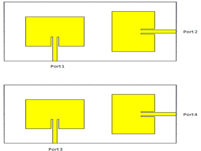
Fig.13. 2X2 MIMO system with four ports
