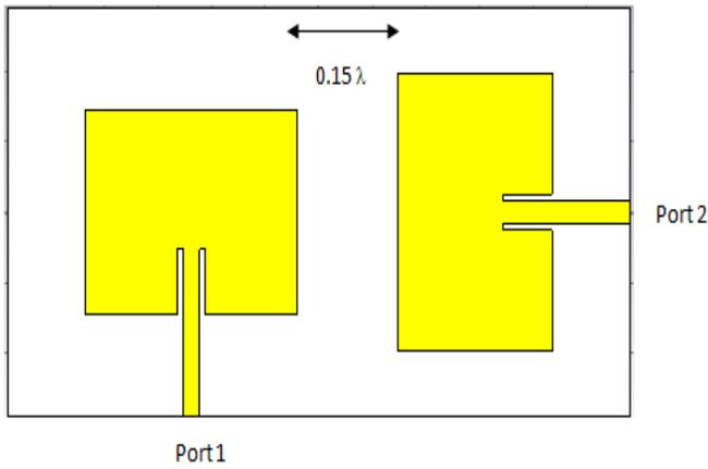
Fig.5. MIMO array of two antenna
