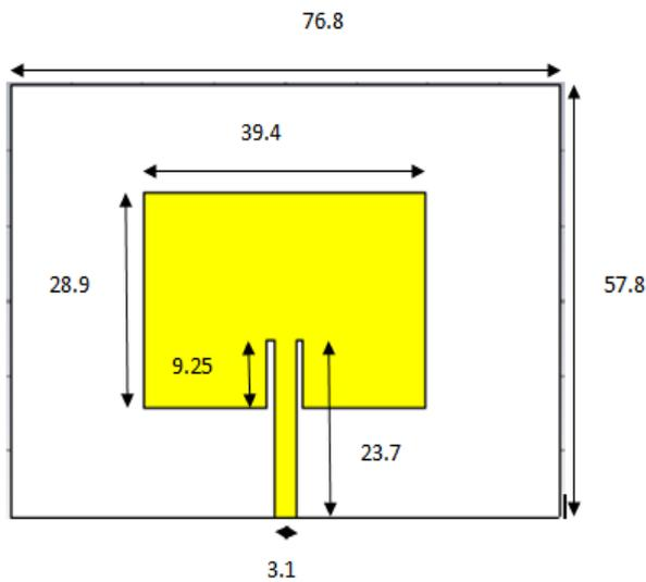
Fig.1. Antenna geometry with dimensions in mm (front view)
