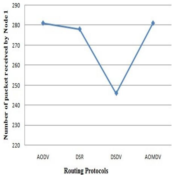
Fig 4. Total number of packet received by node 1 at each routing protocol.
