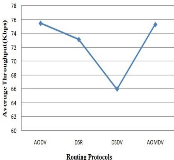
Fig 6. Average throughput at each routing protocol.
