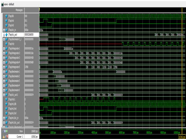
Fig (e) :Simulation of combined multirate filter
