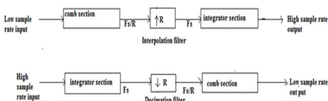
Fig (b): combined interpolation filter and decimation filter( multi rate filter)
