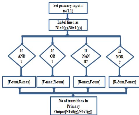
Fig.1.Flow chart to compute transitions in circuit.
