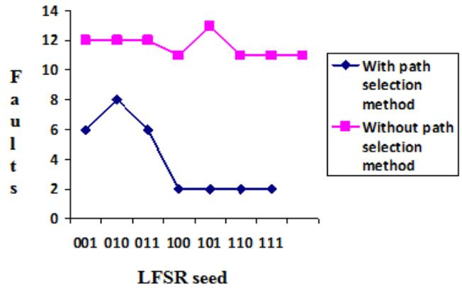
Fig.7.Comparison of faults with LFSR seeds of s298 benchmark circuit
