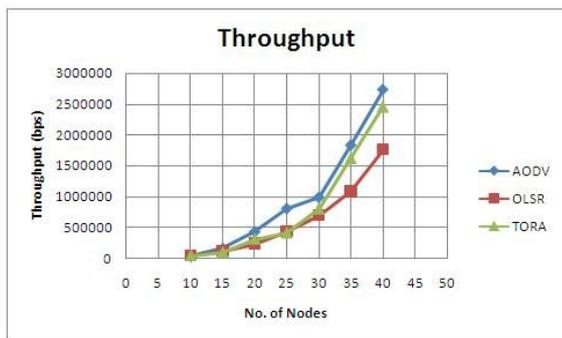
Fig 2: Throughput versus number of nodes
