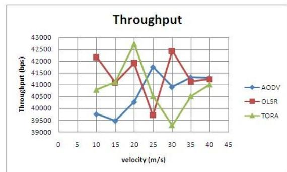
Fig 1: Throughput versus mobility of nodes
