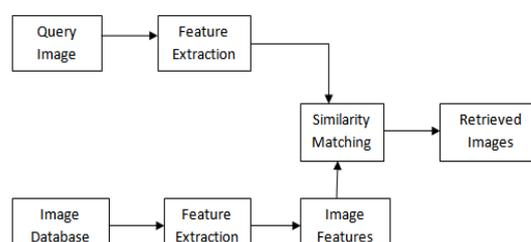
Figure 1: Block diagram of CBIR
