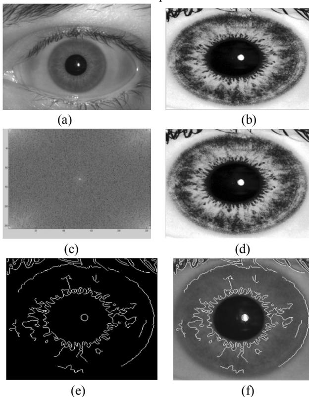
Fig. 5: Different Stage output image in Zigzag collarette boundary localization; (a) Cropped eye image, (b) Image after histogram equalization, (c) Image after 2-D DFT and FFT Shift, (d) Image After inverse FFT, (e) Image after canny edge detection with zigzag collarette detected and located, (f) Collarette boundary is shown in original image.
