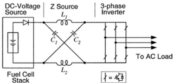
Fig.12. Z-source inverter for fuel-cell applications.
