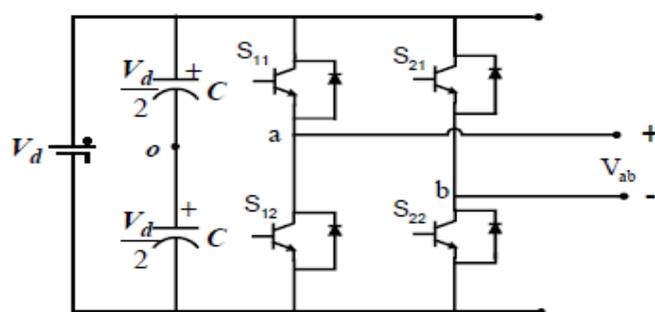
Fig. 3. Single Phase Full-Bridge Inverter.
