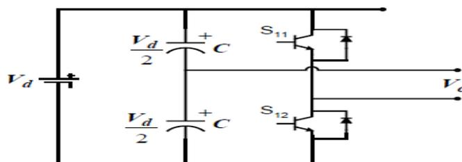
Fig. 4. diagram for Half-Bridge PWM inverter.
