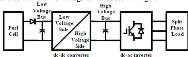
Fig. 2. Block diagram of the fuel cell inverter system
