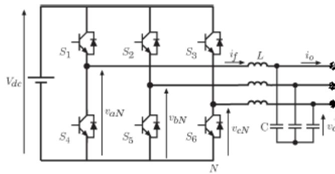
Fig.9. Three-phase PWM inverter with LC filter.
