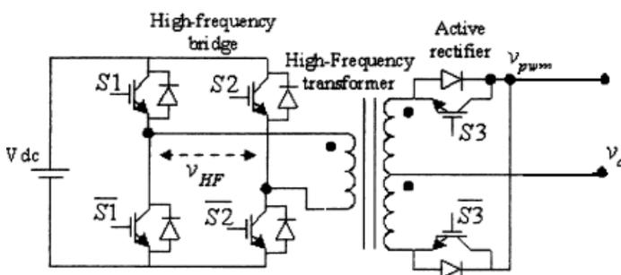
Fig.10. Block diagram of the inverter.
