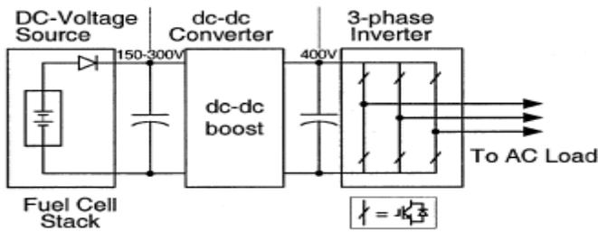
Fig.11. Traditional two-stage power conversion for fuel-cell applications
