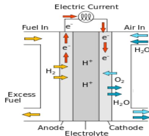
Fig. 1. A basic schematic diagram of a fuel cell
