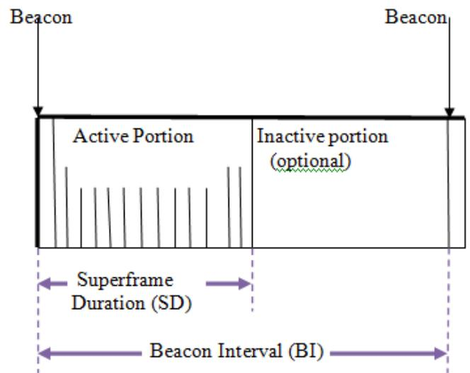
Figure 2. Beacon interval and superframe structure
