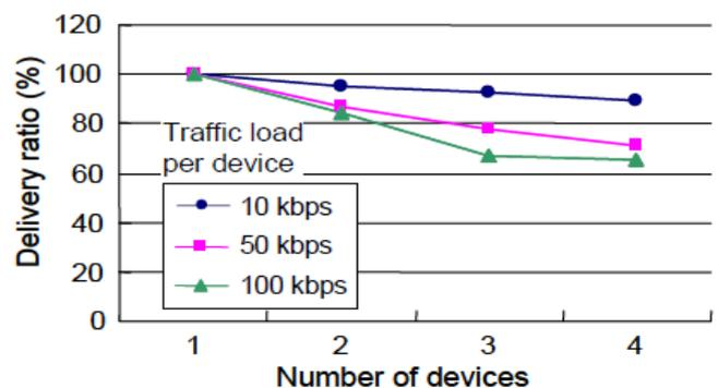
Figure5. Delivery ration of CSMA-CA with varied traffic loads in non beacon-enabled network [8].
