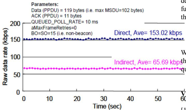
Figure 6. Raw data rate for direct and indirect transmission for non beacon-enabled network [8].
