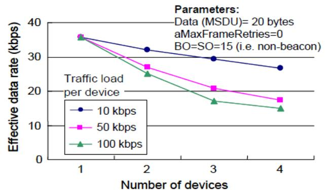
Figure 4. Effective data rate of CSMA-CA with varied traffic load in non beacon-enabled network [8].
