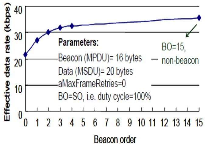
Figure 3. Effective data rate in beacon-enabled network [6]
