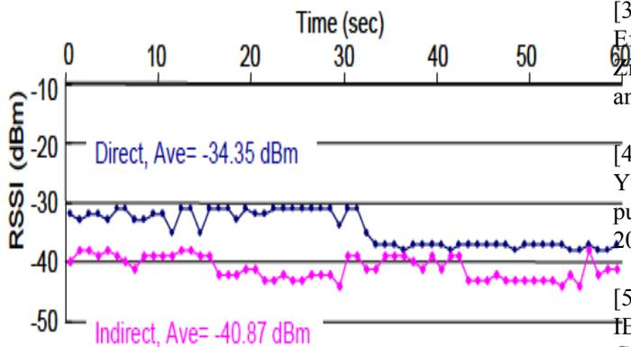
Figure 7. RSSI value for direct and indirect data transmission in non beacon-enabled network [8].
