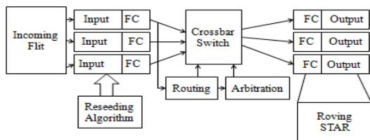
Figure 2. Fault Tolerant NoC router
