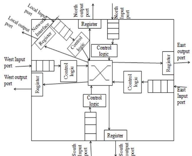
Figure 1. Typical NoC router architecture.
