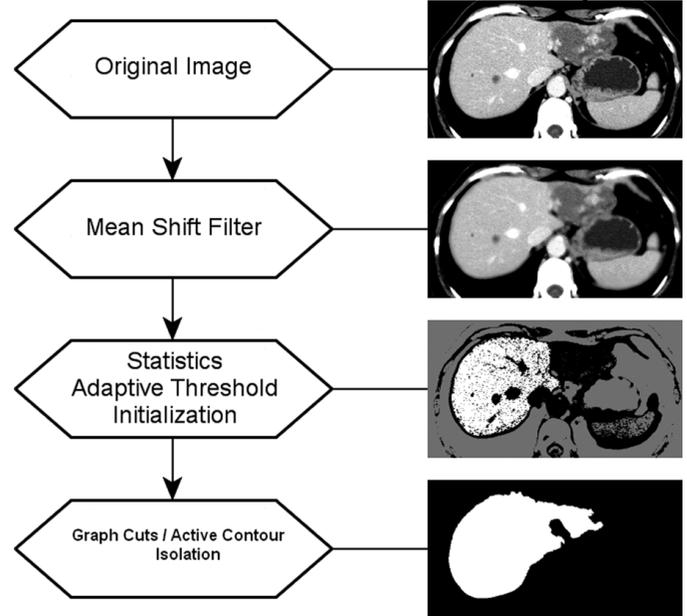
Figure 1. Flowchart of the automatic liver initialization method.
