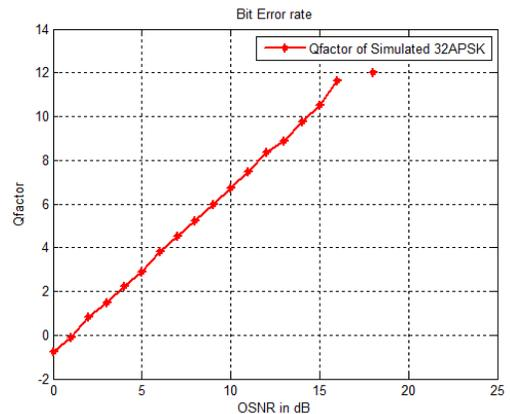
The Q-factor value is very important for the modulation technique, it implies that how efficient our system is. Here Q value is calculated with OSNR value hence it indicates that loss is reduced than existing paper.
