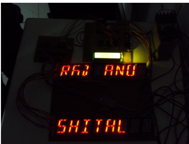
Figure 7. Display Received Message on Alphanumeric Display Board
