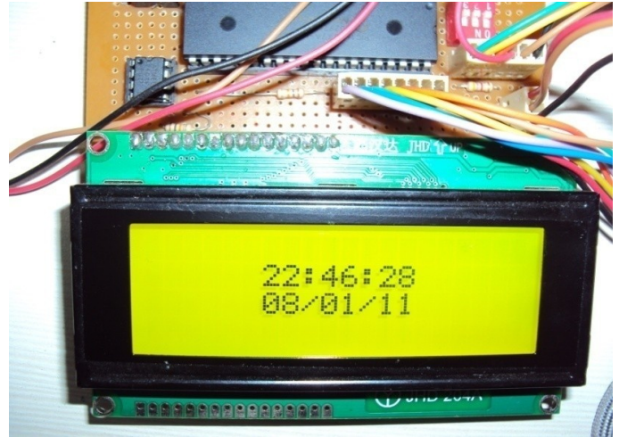
Figure 8. Display Real time clock and date
