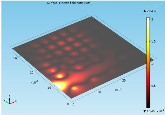
Figure 3: Distribution of electric fields z component (EZ) for 1.2 $\mu\text{m}$
