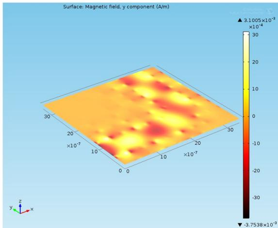
Figure 6: Distribution of magnetic fields y component (EZ) for 1 $\mu\text{m}$
