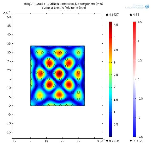
Figure: 9 Self-collimated beam for 1.2 $\mu$ m wavelength
