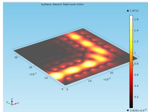
Figure 2: Distribution of electric fields  $z$  component ( $E_z$ ) for  $1\mu\text{m}$
