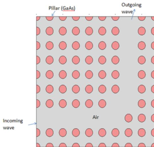
Figure 1: Schematic of a 2-D pillar-type PC consisting of a square lattice
