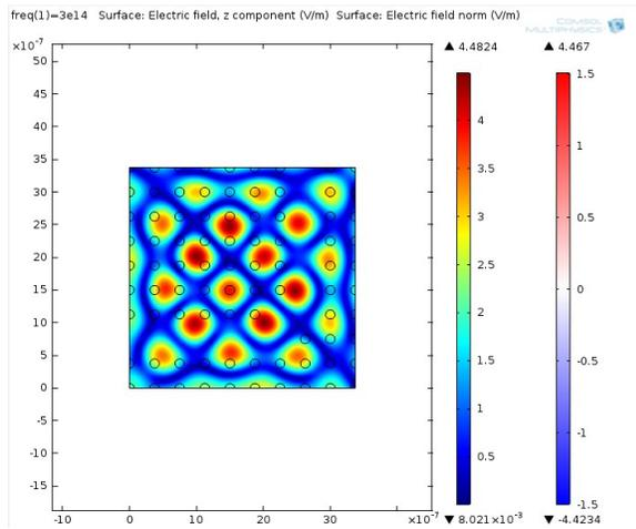
Figure:8 Self-collimated beam for 1 $\mu$ m wavelength
