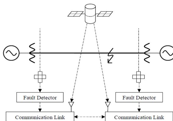
**Fig 1 GPS satellite used to synchronize fault detection timing**
