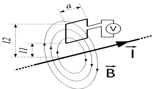
Fig. 2. Magnetic loop for measurement of current along a conductor.
