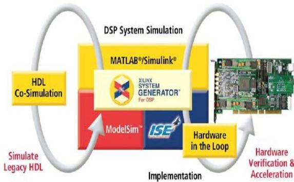
Fig-1 .Design flow of XSG system
