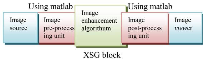
Fig -1. Design flow of hardware implementation of image enhancement.
