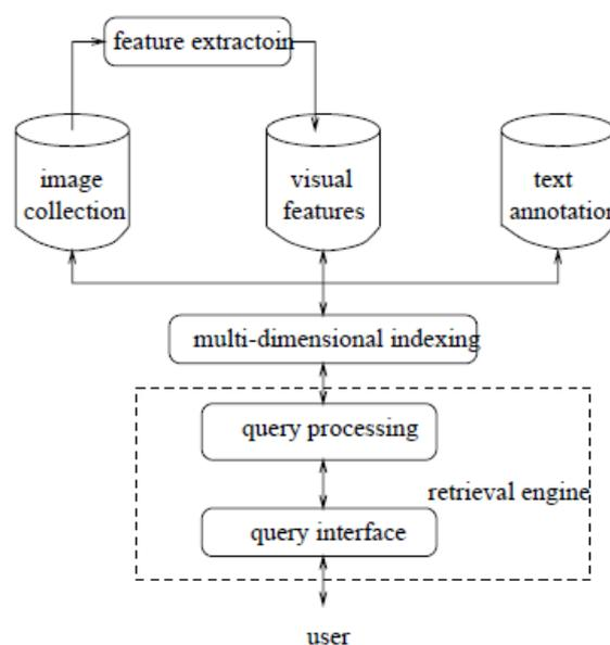
Fig 1: Architecture of Image Retrieval System
