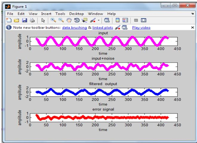
Fig 3.1: Output Plot of LMS Algorithm
