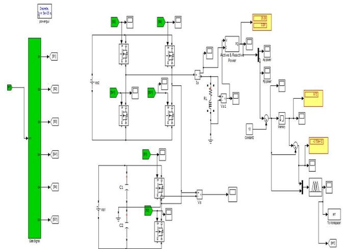
Fig 6. Simulation Circuit For Reactive power control
