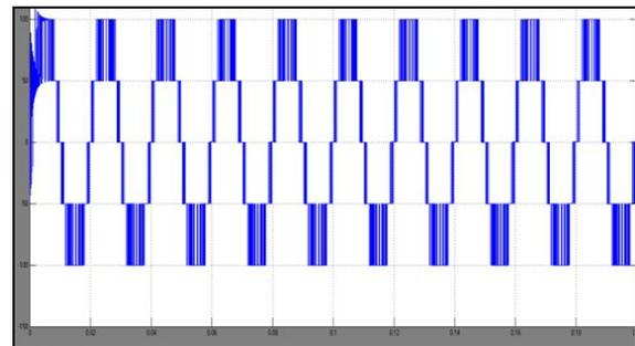
Fig 7. Five level inverter output.
