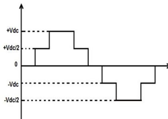
Fig 3. Five level inverter output
