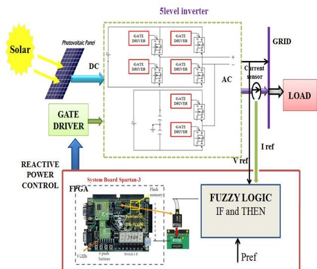
Fig 1. Block diagram of Proposed Mechanism
