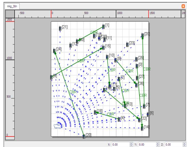
Fig. 1. A Scenario for AODV and DSR Routing Protocols (on 30 Nodes).
