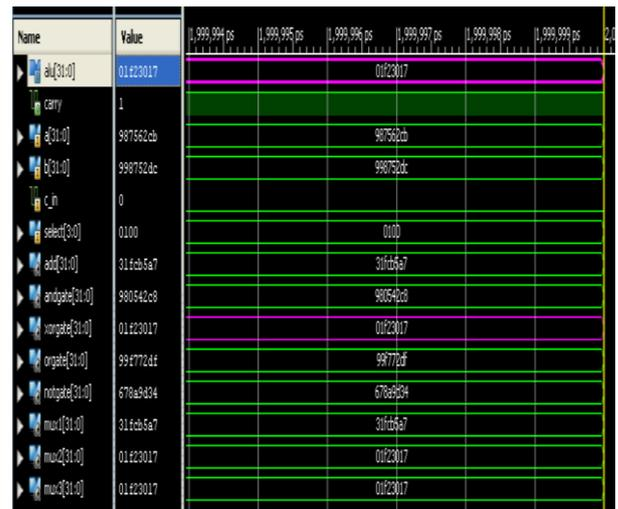
Figure 5: Simulation Results for 32-bit ALU Chain Structure
