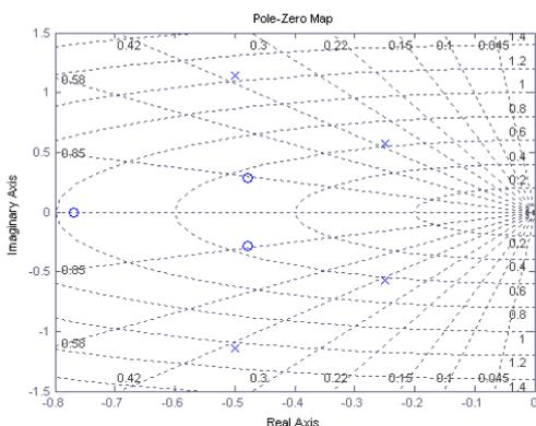
Fig. 5. Diagram placing poles and zeros of the transfer function  $\tilde{W}_V^{\delta_{PB}}$
