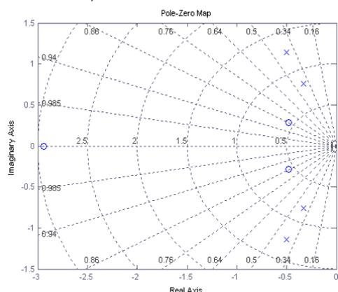
Fig. 6. Diagram placing poles and zeros of the transfer function  $\tilde{W}_g^{\delta_{PB}}$
