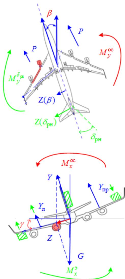
Fig. 8. The stabilizing forces and moments Boeing 747
