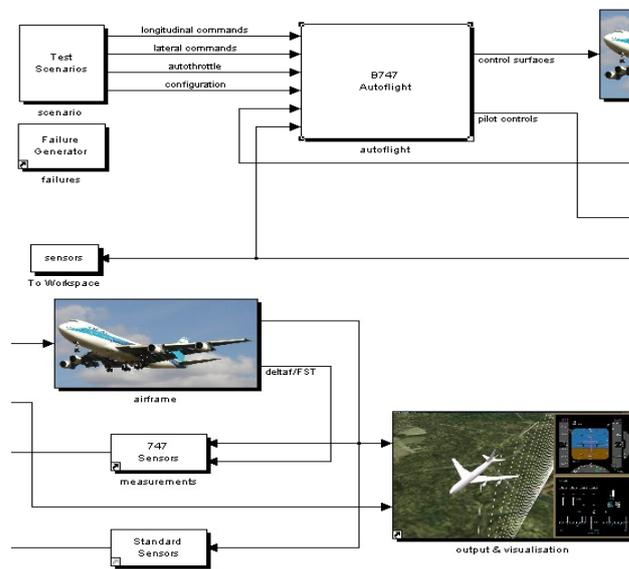
Fig. 9. The generalized structure of software, which includes the following blocks: autoflight - block automatic flight control systems, airframe - the Boeing 747 model, scenario - Action Plan (unit reconfiguration), sensors sensors; failure generator - generator of typical failures [15].
