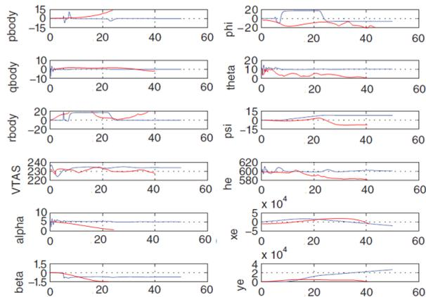
Fig. 10. The results of mathematical modeling of an emergency, where: Crane line - without reconfiguration, the blue line - using reconfiguration upravlyaniya plane.
