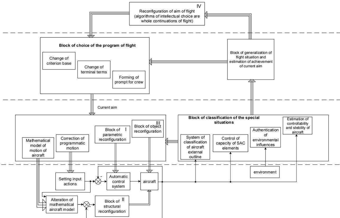
Figure 2. Flow diagram of reconfigured control system of aircraft in the conditions of origin of exception condition on wing
