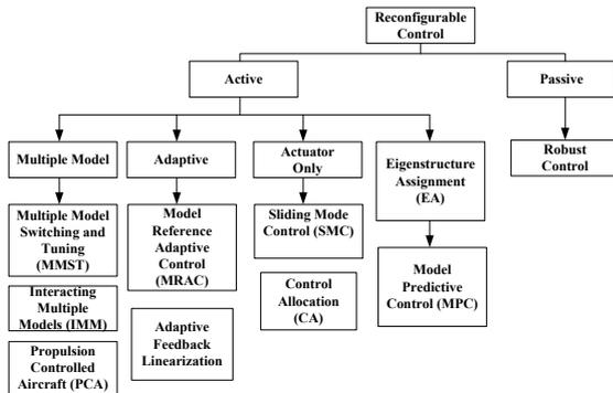
Figure 1. Classification of approaches to reconfigurable flight control
