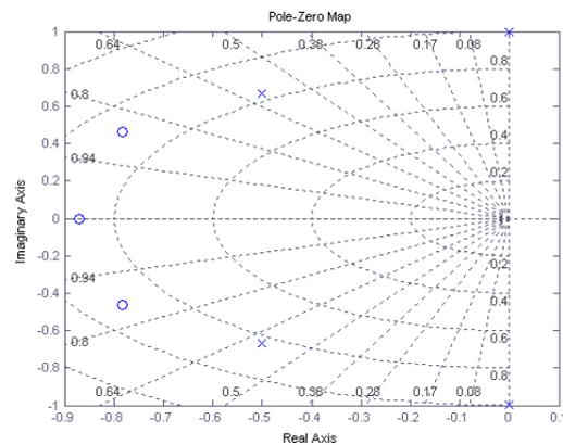
Fig. 3. Diagram placing poles and zeros of the transfer function  $\tilde{W}_V^P$
