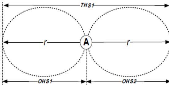
Fig. 1. Illustration of a two-hop set, where an ellipse represents an OHS such that all nodes inside one ellipse can directly communicate with each other, with node A as a reference.
