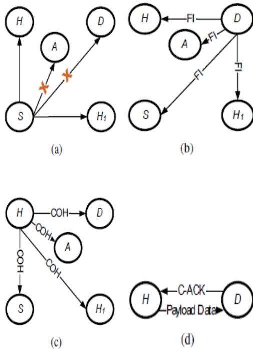
Fig. 3. Information exchanges in the CAH-MAC: a) The direct transmission; b) Neighboring nodes detect transmission failure after examining the FI from the destination; c) Helper node H, offers cooperation; d) Helper node H, re-transmits the packet that failed to reach the destination after receiving a cooperation acknowledgement from the destination.(ref. 2).
