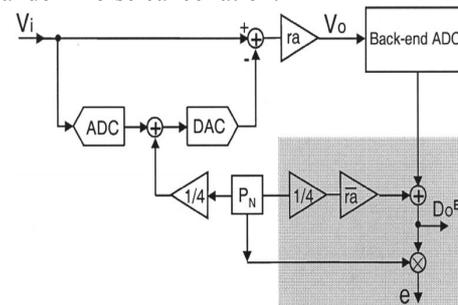
Figure 2: Background Equivalent Calibration with Radix Extraction
