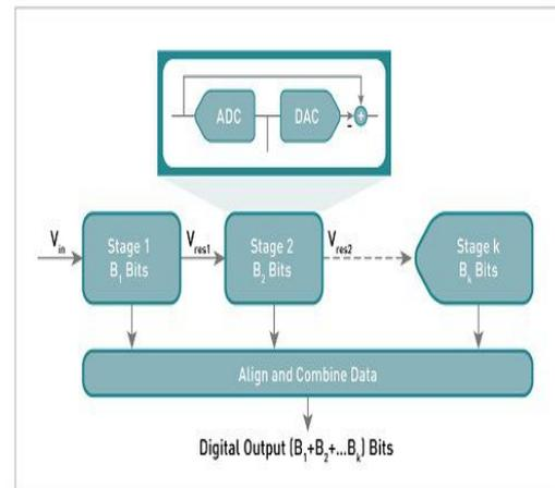
Figure 1: Block Diagram of Pipelined ADC
