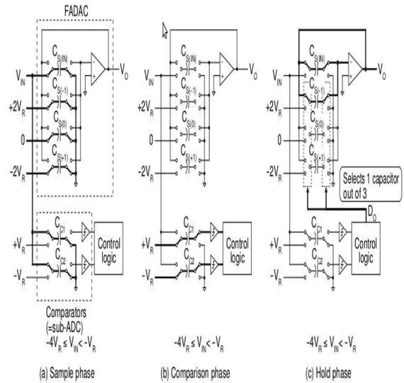
Figure 5: Block Diagram FADAC
