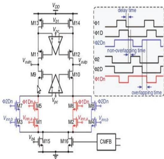
Figure 3: Switch Embedded Op-amp Architecture
