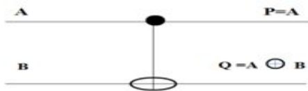
Fig 2(b): Quantum implementation of Feynman gate
