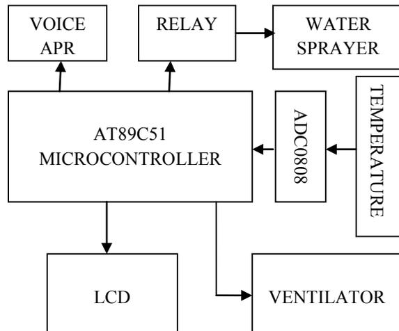
Fig.1.Block diagram of transmitter node
