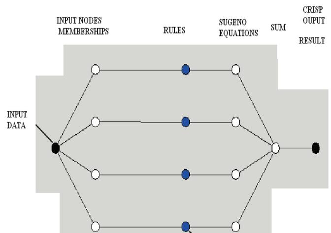
Fig. 9b. An ANFIS network uses input data and output result and finds the Fuzzy Inference System model for such data pair. One single input and one output model shown.
