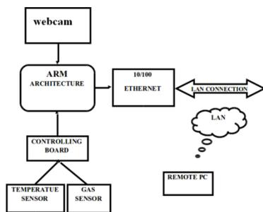
Fig.1 Block Diagram of the Total System
