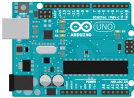
Fig.3 Arduino microcontroller board
