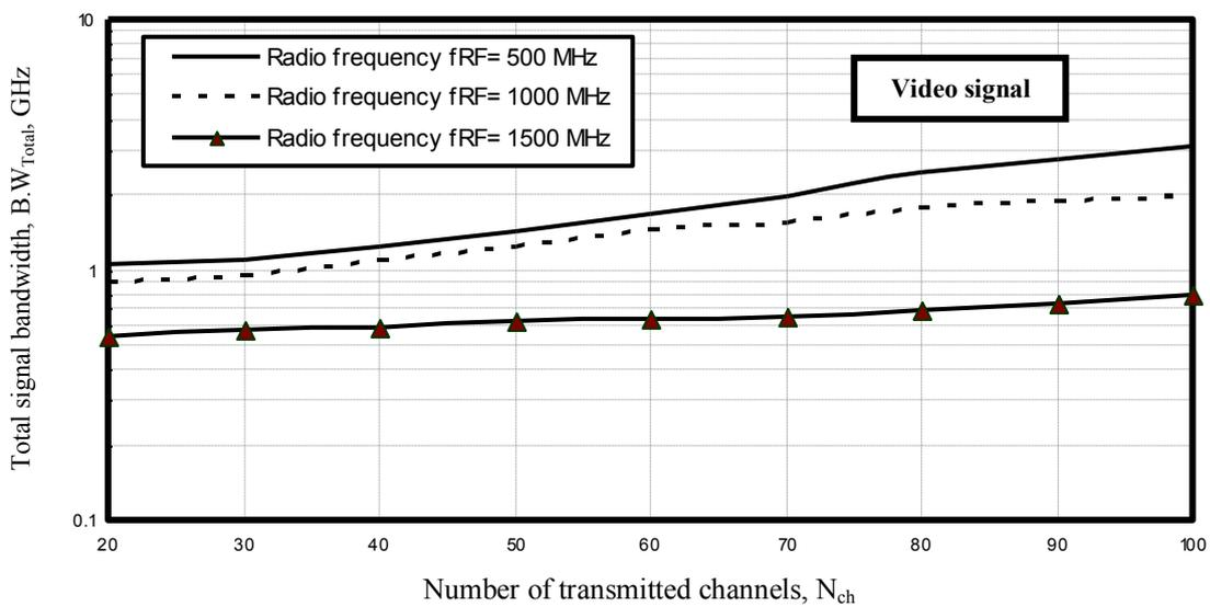
Fig. 7. Variations of the total system signal bandwidth against number of transmitted channels at the assumed set of the parameters.
