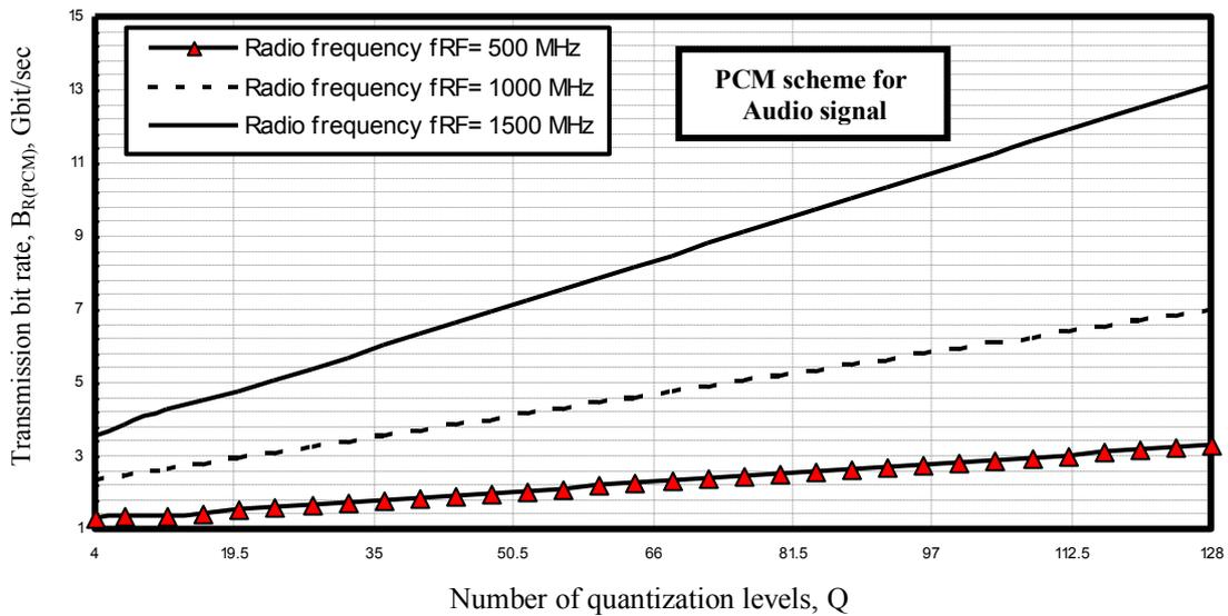
Fig. 12. Variations of the transmission bit rate against number of quantization levels at the assumed set of the parameters.
