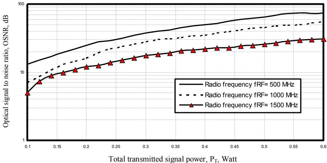
Fig. 1. Variations of the optical signal to noise ratio against total transmitted signal power at the assumed set of the parameters.
