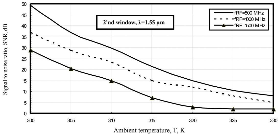
Fig. 2. Signal to noise ratio in relation to ambient temperature and operating signal radio frequency at the assumed set of the operating parameters.
