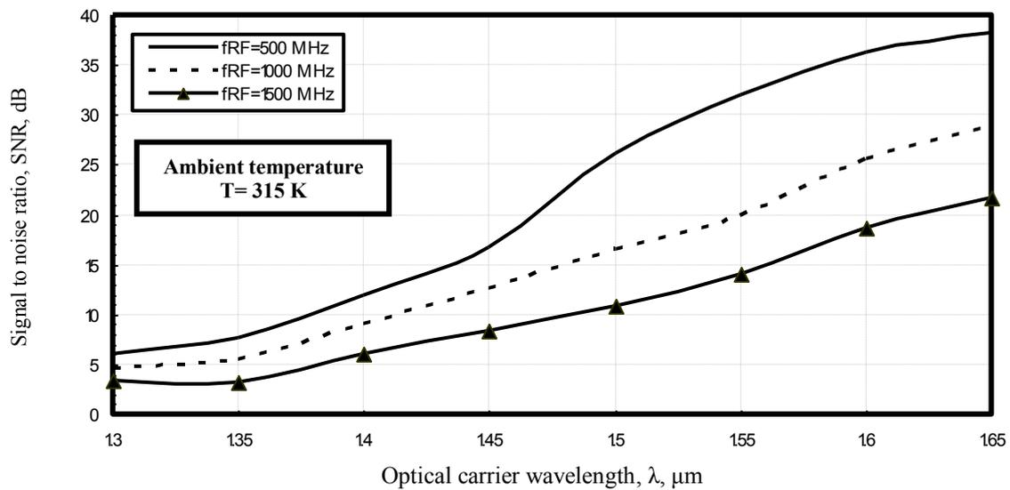
Fig. 4. Signal to noise ratio in relation to optical carrier wavelength (with  $T=315\text{ K}$ ) and operating signal radio frequency at the assumed set of the operating parameters.
