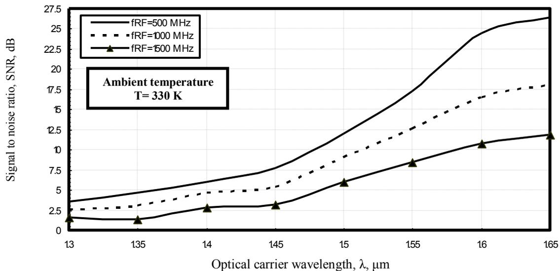
Fig. 5. Signal to noise ratio in relation to optical carrier wavelength (with  $T=315\text{ K}$ ) and operating signal radio frequency at the assumed set of the operating parameters.
