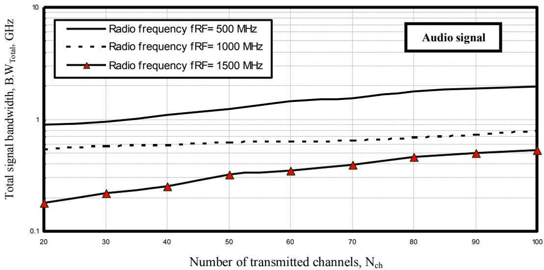
Fig. 6. Variations of the total system signal bandwidth against number of transmitted channels at the assumed set of the parameters.
