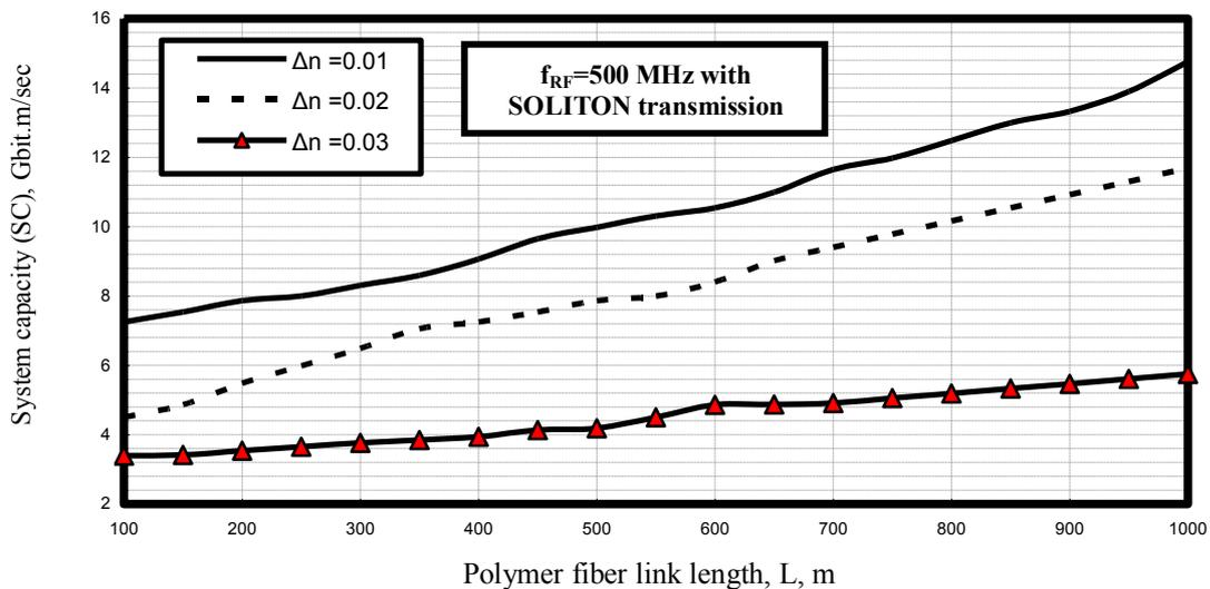
Fig. 11. Variations of the system transmission capacity against polymer fiber link length at the assumed set of the parameters.
