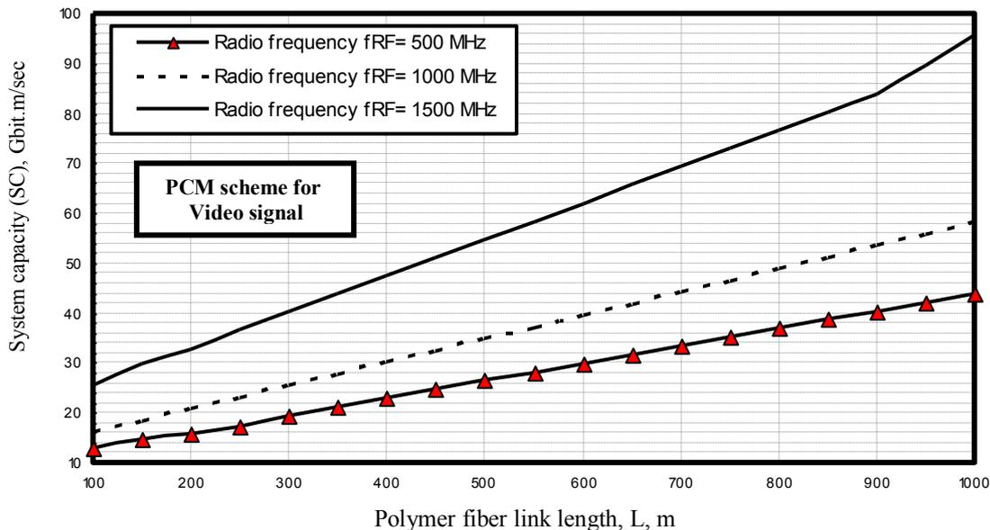
Fig. 15. Variations of the system transmission capacity against polymer fiber link length at the assumed set of the parameters.
