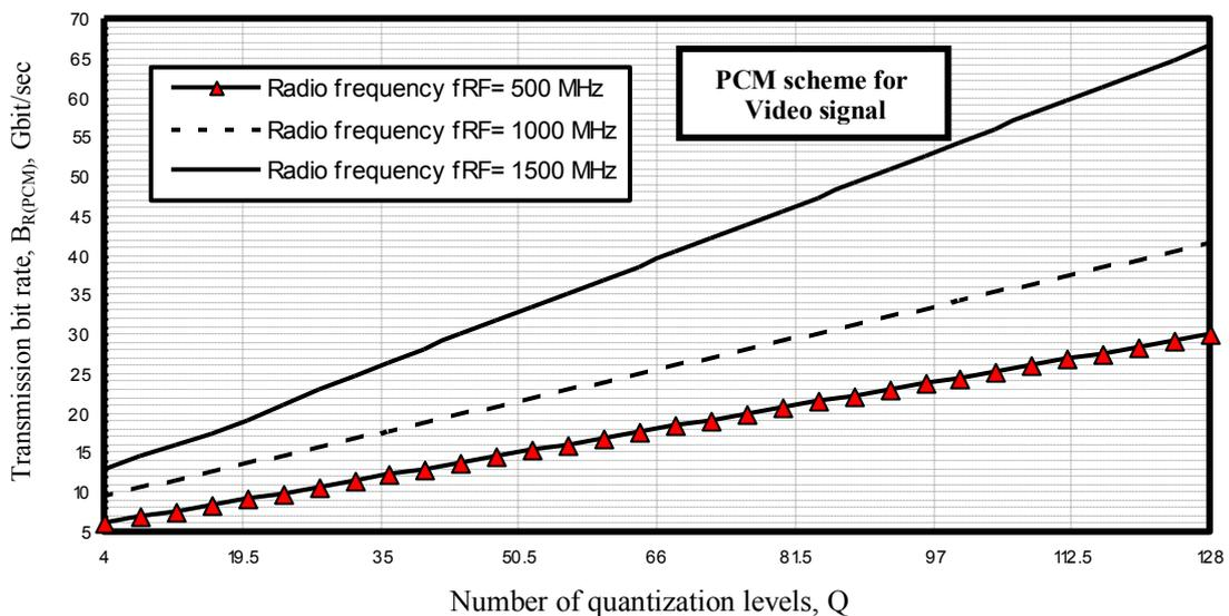
Fig. 13. Variations of the transmission bit rate against number of quantization levels at the assumed set of the parameters.
