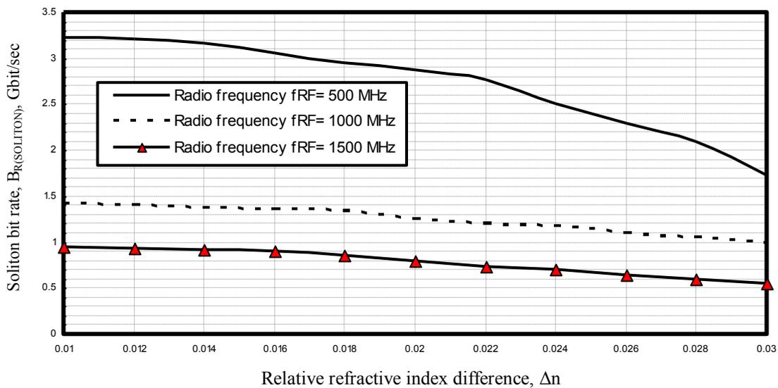
Fig. 8. Variations of the Soliton transmission bit rate against relative refractive index difference at the assumed set of the parameters.
