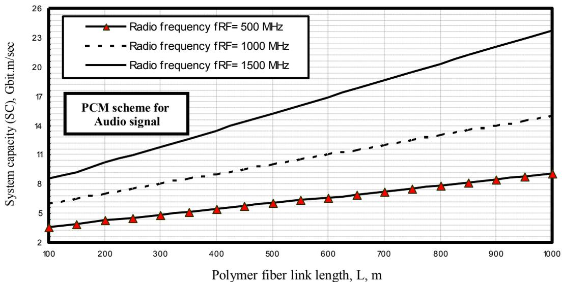
Fig. 14. Variations of the system transmission capacity against polymer fiber link length at the assumed set of the parameters.
