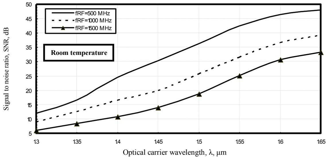
Fig. 3. Signal to noise ratio in relation to optical carrier wavelength with room temperature and operating signal radio frequency at the assumed set of the operating parameters.
