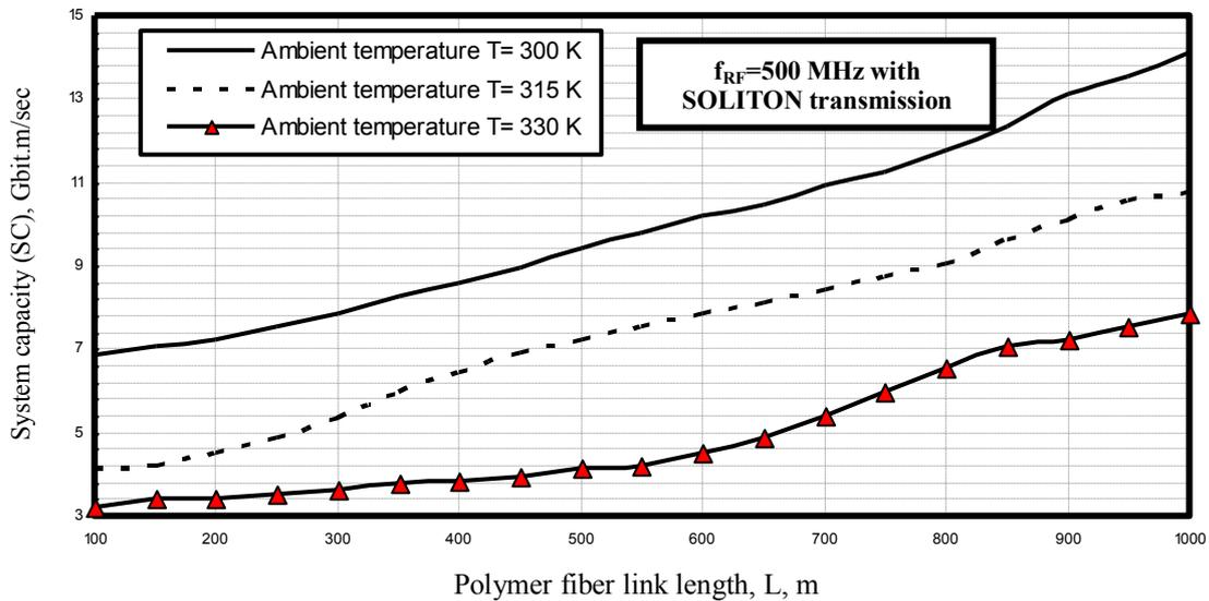
Fig. 10. Variations of the system transmission capacity against polymer fiber link length at the assumed set of the parameters.
