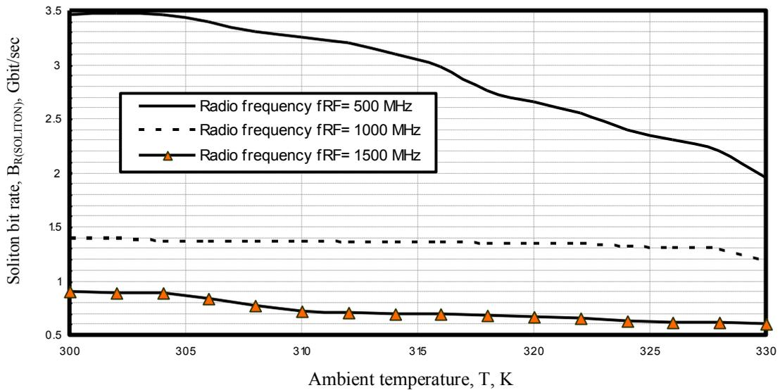
Fig. 9. Variations of the Soliton transmission bit rate against ambient temperature at the assumed set of the parameters.
