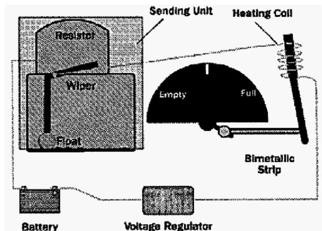
Figure1. Traditional Fuel Measurement System [1]
