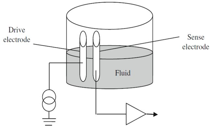
**Figure2. Capacitive Level Sensing [2]**
