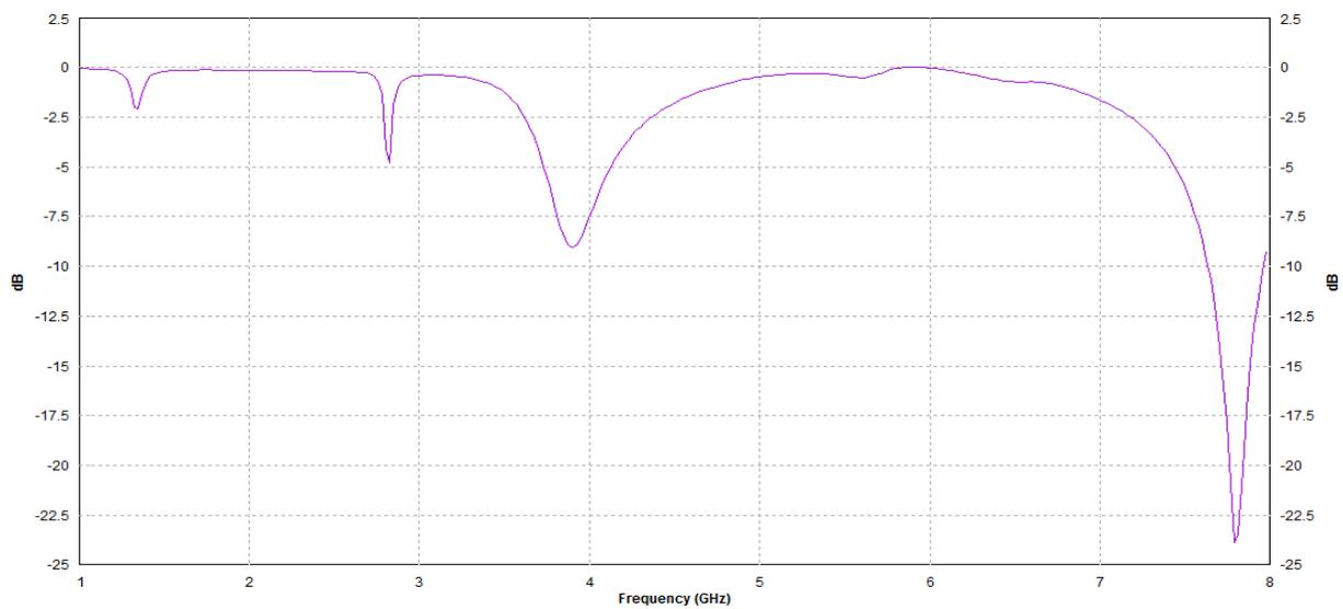
Fig. 9  $S_{11}$  vs Frequency (3<sup>rd</sup> Iteration)
