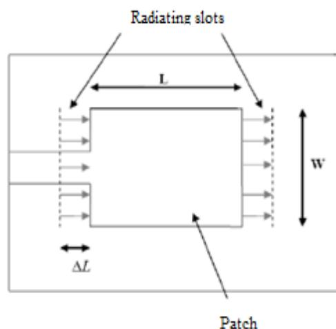
Fig. 2 Top view of antenna
