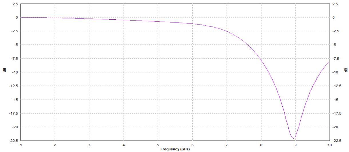
Fig. 7  $S_{11}$  vs Frequency (1<sup>st</sup> Iteration)
