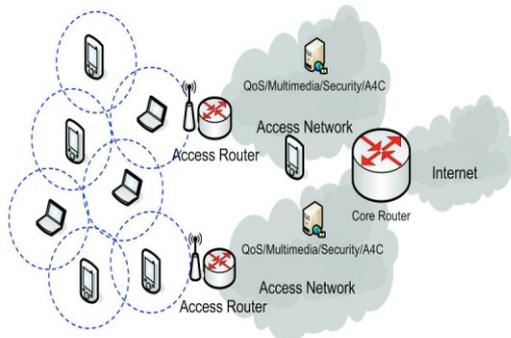
Fig. 1: Example of wireless network with Permanent access points
