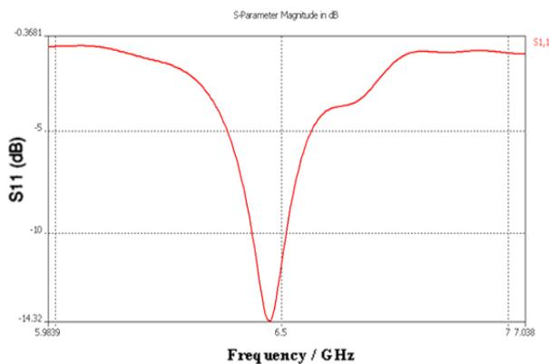
Fig5. S11 of reference antenna with diode OFF
