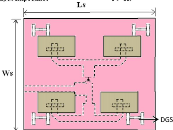
Fig2 Structure of frequency reconfigurable reference antenna.
