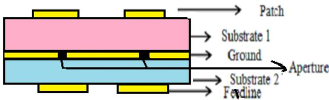
Fig.1. Side view of the proposed antenna.
