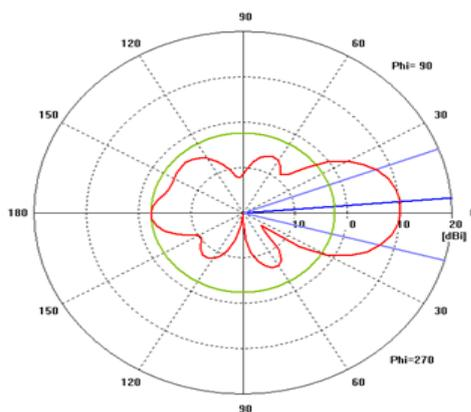
Fig 6. Farefield pattern when diode is OFF of reference antenna CASE 3. With DGS diode ON
