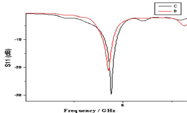
Fig11.S11 of the frequency reconfigurable antenna with DGS and diode OFF
