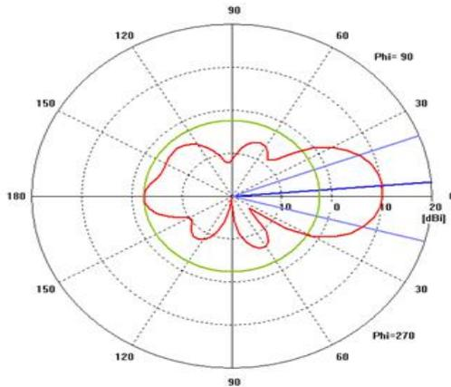
Fig10.farfield of the frequency reconfigurable antenna with DGS and diode OFF
