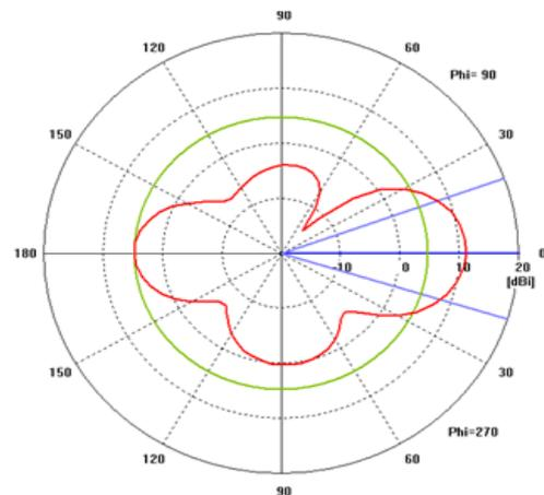
Fig8. farfield pattern of the frequency reconfigurable antenna with DGS
