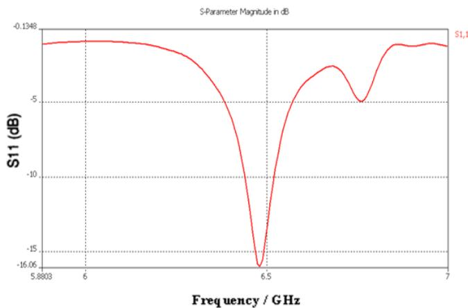
Fig9. S11 of the frequency reconfigurable antenna with DGS and diode OFF
