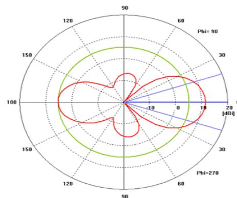
Fig4.Farfield pattern of the reference antenna
