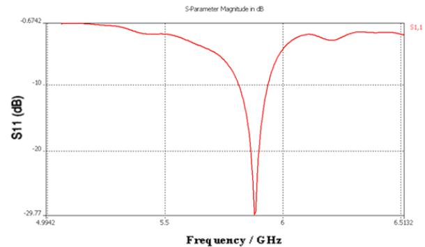
Fig7. S11 of frequency reconfigurable antenna with DGS Farfield pattern of the antenna is shown in fig8, it's main lobe magnitude is 11.1 dBi, direction of the maximum radiation is 0 degree and Side lobe magnitude is -6.2 dB. In this case radiation efficiency of the antenna is improved as compared to the reference antenna.
