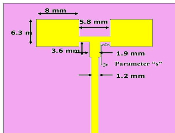
Fig.1 Reference Antenna layout without EBG pattern
