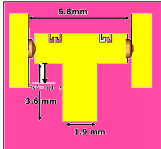
Fig.3 Magnified view of the feedline of antenna variant-1
