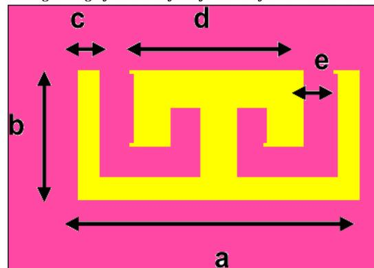
Fig. 4 Single EBG pattern-1 etched on feedline of antenna variant-1
