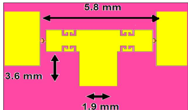
Fig.5 Magnified view of the feedline of antenna variant-2
