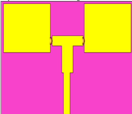
Fig 2 shows the Magnified view of the reference antenna when there is no EBG pattern is introduced.
