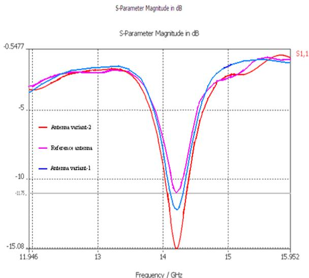
**Fig.11 comparison between reference antenna, antenna variant-1 and antenna variant-2 when both diodes are ON.**
