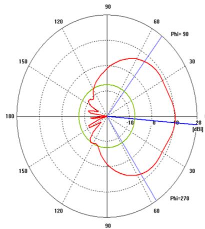
Fig.9 Farfield pattern Abs (Theta) of the antenna array antenna variant-1 EBG pattern when both diodes are ON
