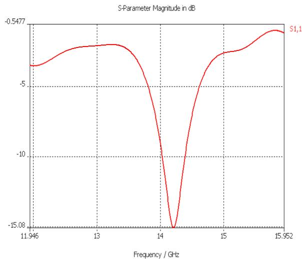
**Fig.10 shows the S11 graph of the antenna variant-2 EBG pattern when both diodes are ON**
