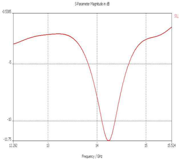
Fig.6 S11 graph of the antenna array when there is no EBG pattern is applied.
