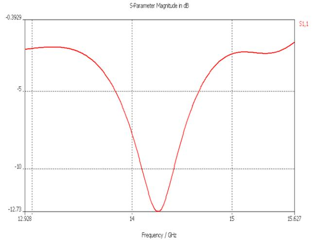
Fig.8 S11 graph of the antenna array antenna variant-1 EBG pattern when both diodes are ON
